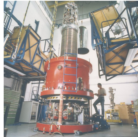
5.5 MeV Van De Graaf Injector Hahn-Meitner Institute, Berlin (ECR ion source at the terminal)
